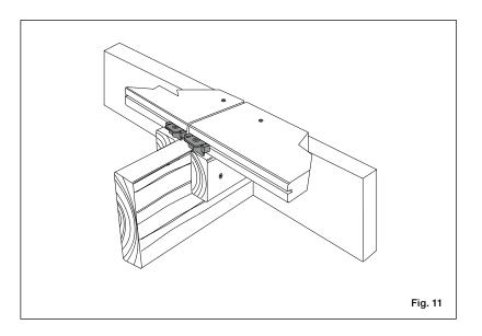
**Step 3** On the other side of the board, place a Stowaway hidden fastener into the groove and center on the joist (Fig. 12). Install the preset screw at a 90° angle through the Stowaway fastener and drive flush. Do not over-tighten. The fastener wings must remain level with the joist for the next board to fit correctly (Fig. 13).
