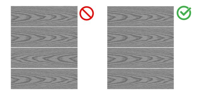
To keep gaps lined up, you must build all sections of a split deck at the same time. This will allow you to adjust for natural variation in board width as you go. Snap 1 line to start the decking then reference with a measurement every 2 or 3 rows off the original line.
