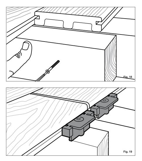
**Step 8** Repeat the process for each board until the outside edge of the final board is fastened with screws. Use fascia to conceal the board profile and inhibit board movement over time. Please refer to the fascia installation instructions for the approved fastening methods for fascia boards.
