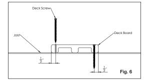
B) Standard Surface Fastening: Use two fasteners per deck board at each joist. It is required that screws be placed 0.50" from both edges to ensure screws are in the thickest lobed area.
