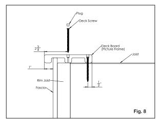
D) Board End Fastening: For any decking where two boards meet end-to-end over a joist, you must add additional blocking (fig. 9/10). It is required that screws be placed 0.50" from both edges to ensure screws are in the thickest lobed area. Screws must also be placed at least 1-1/2" from the cut end of the deck boards. Be careful to not to over-tighten screws near board ends.
