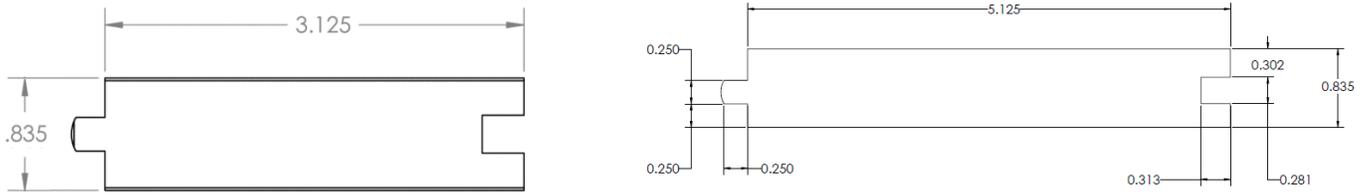
FIGURE 4 – DECKORATORS® PORCH PROFILES (TONGUE AND GROOVE)
