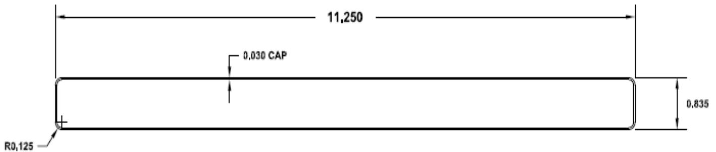
FIGURE 8 – 11.25" DECKORATORS® VOYAGE VARIED-PLANK DECKING
