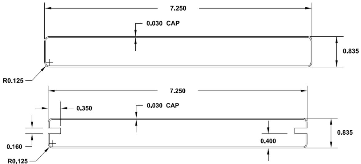
FIGURE 6 – 7.25" DECKORATORS® VOYAGE VARIED-PLANK DECKING
