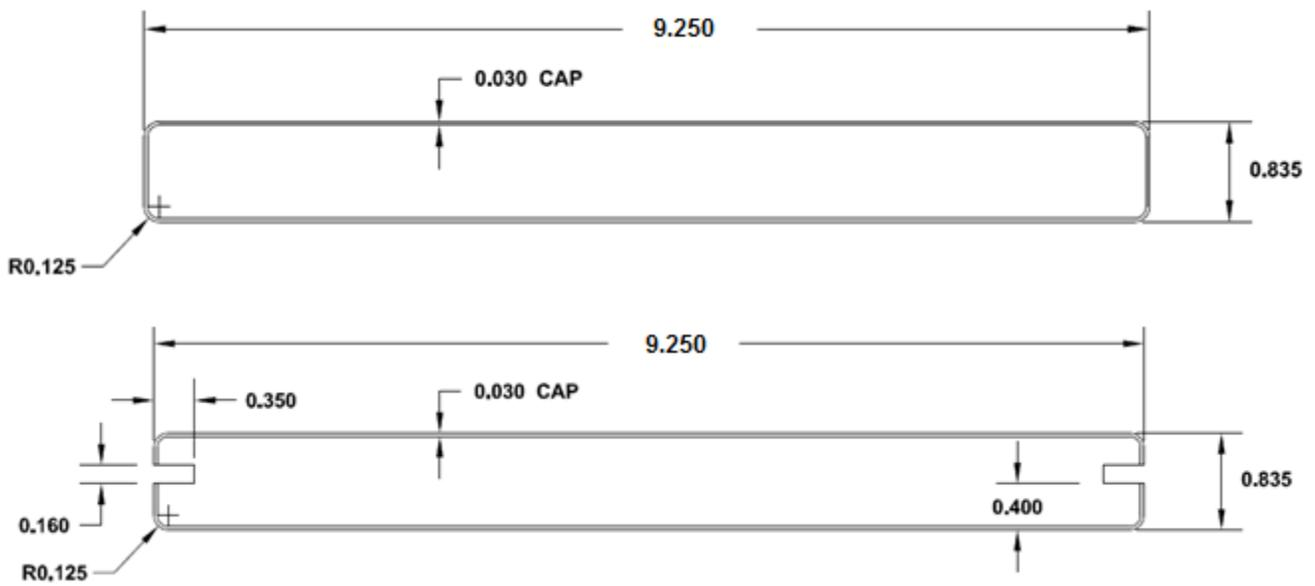
FIGURE 7 – 9.25" DECKORATORS® VOYAGE VARIED-PLANK DECKING
