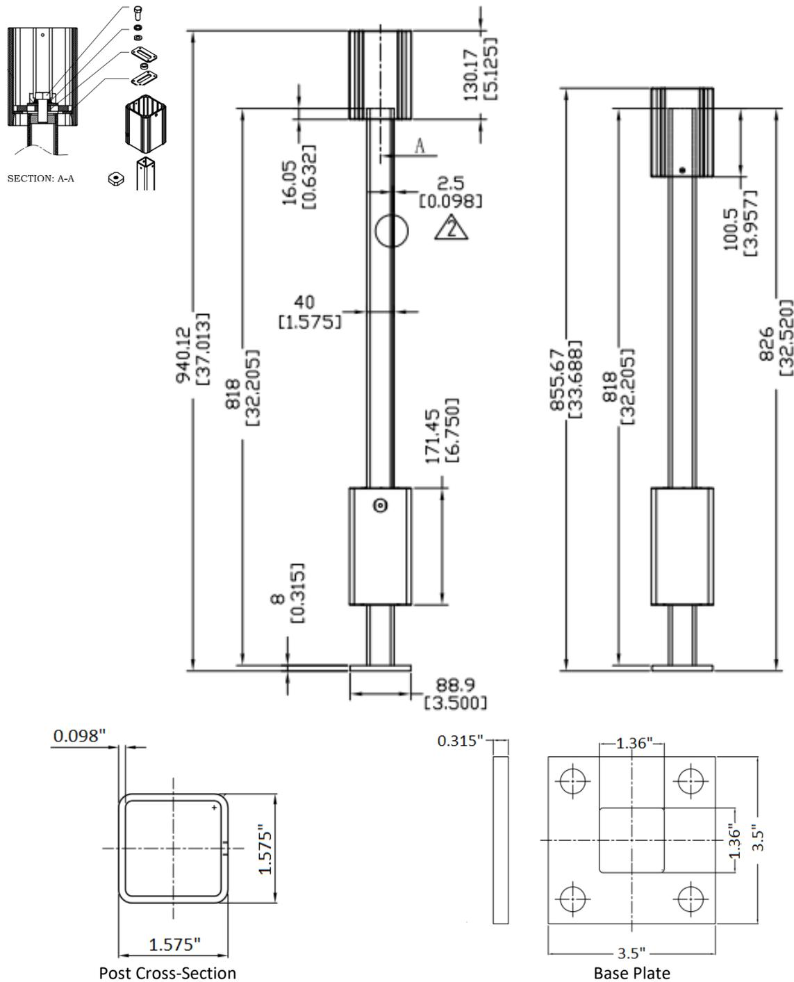
Figure 3 – Advantage Plumb Perfect Post Mount System
