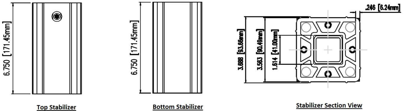
Figure 7 – Post Stabilizers for Atlas-Pro and Advantage V2
