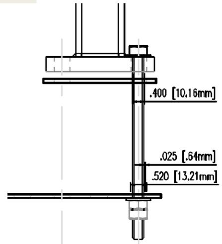
Plate Installation Configuration
