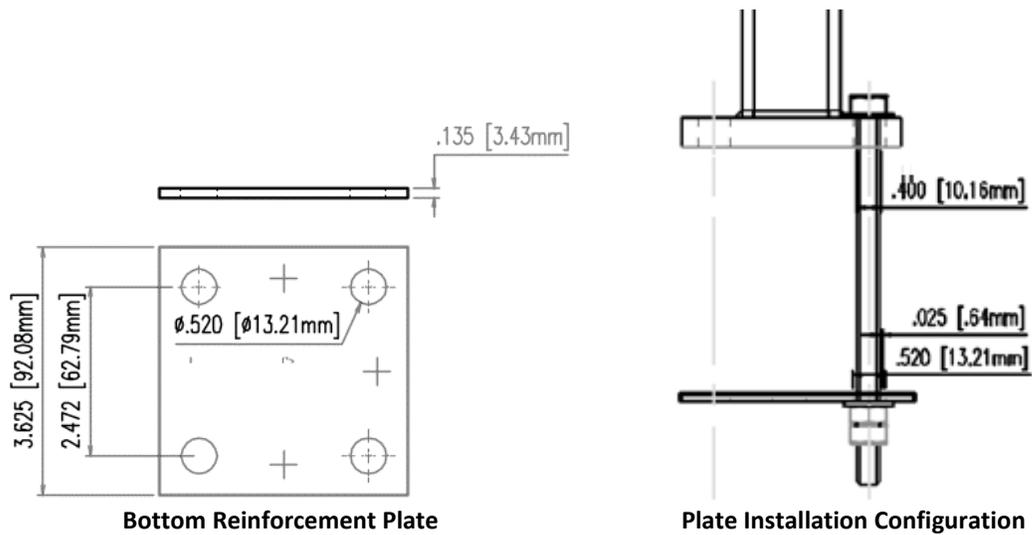
Figure 6 – Post Mount Installation to Wood blocking using 3-5/8 inch Reinforcement Plates
